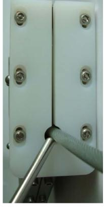
The 8 mm finger rod must not fit into the notch!
