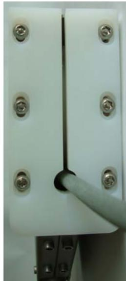
For a proper course of the pulley and to avoid tilting or abrasion of the rope, the lateral impact plates of the pulley can be vertically adjusted ( included in delivery: screw driver Torx TX 30 with drill for pin – K&K item-Nr. 3490080)
