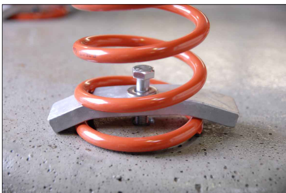
3 x screw connection compression spring/spring holder on form block consisting of: hexagon head screw M12x50-DIN931-zinc-plated; washer \phi 13-DIN125-zinc-plated;
