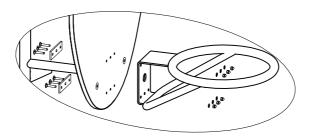
button head screw DIN 603-M8x45-A2; washer DIN 125-Ø8,4-A2; safety cap nut DIN 986-M8-A2.
