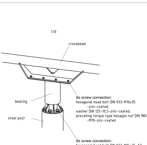
8x screw connection: hexagonal head bolt DIN 933-M16x35-A2; washer DIN 125-17-A2;
