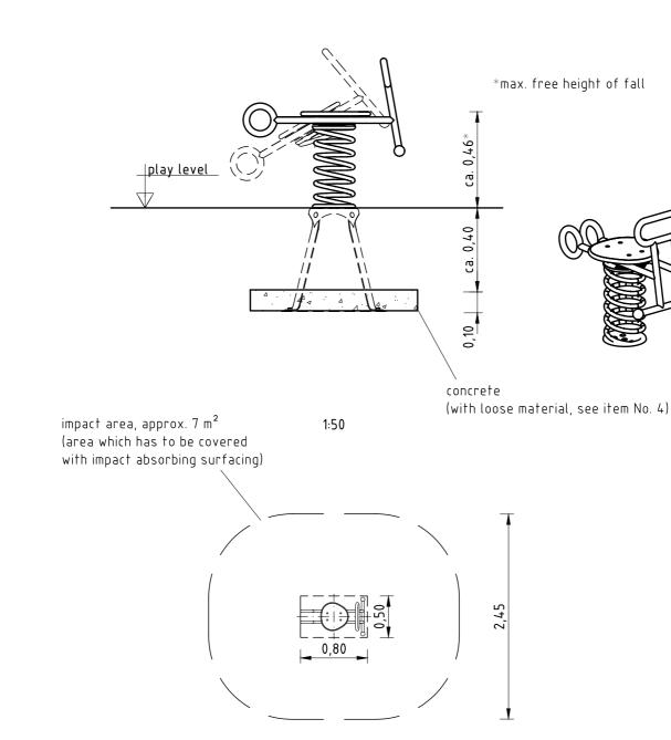
1. Assign a location for the equipment considering the impact area/(falling) space requirements.
