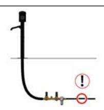
Remove black plastic plugs from the K&K valve combination (= a total of 3) or, where appropriate, uninstall K&K valve combination entirely.
