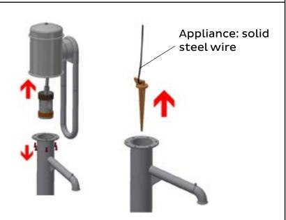
The remaining water between pump and valve combination pours out of the outlets opened before.
